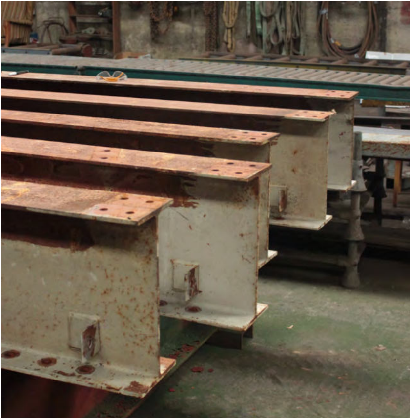
Reclaimed Structural Steel Components in Portal Power's premises in Kenton, Suffolk.
