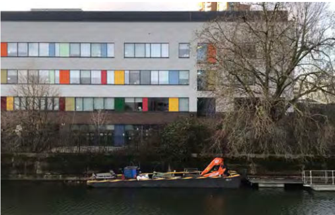
Dumb barge customized with roll-on roll-off equipment, crane and generator.
